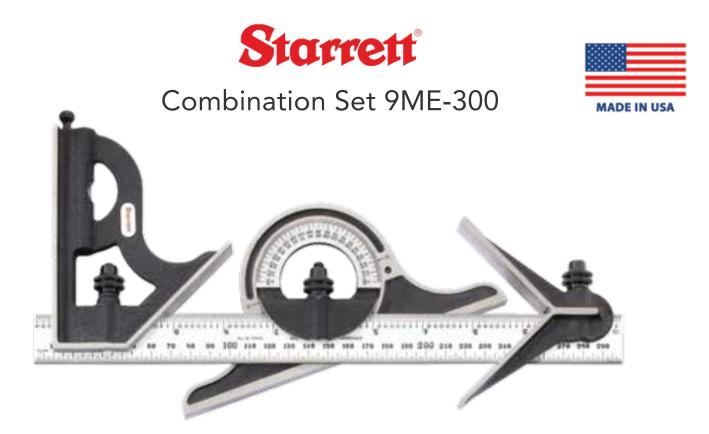
The Starrett 300mm and 11-3/4" Combination Set with Square features a reversible lock bolt, scriber, spirit level in both square head and protractor head, direct reading double 180° protractor scale, and hardened steel, and photo-engraved blade. The combination set includes a cast iron head with black wrinkle finish. 300mm / 11-3/4", Metric/Imperial, Regular Blade finish.
