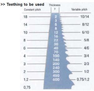
Note : Variable pitch can help to reduce vibrations coming from the resonance sometimes generated by a constant pitch.
